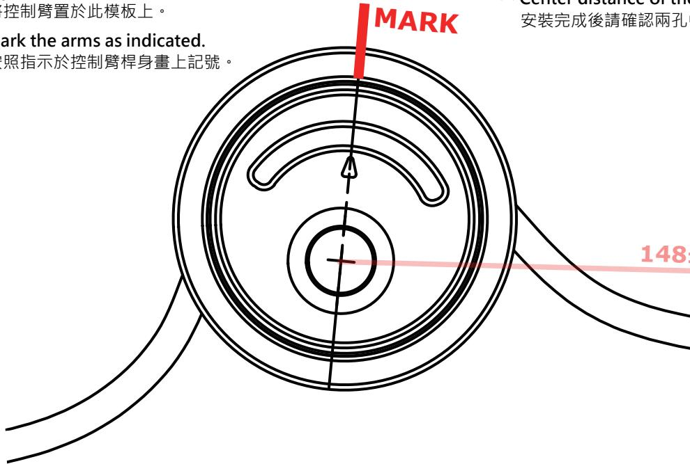
4. Align the marks and press the bushings into the arms.
