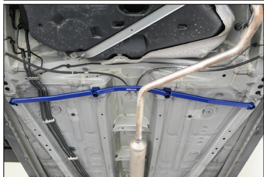
Illustration of installed state 安裝完成示意圖
