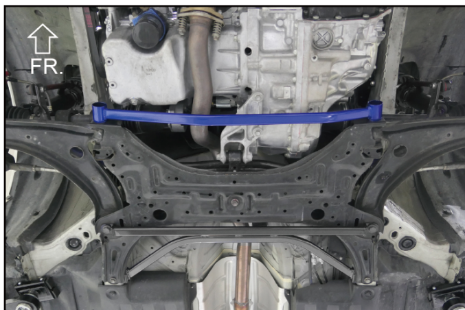
Illustration of installed state 安裝完成示意圖
