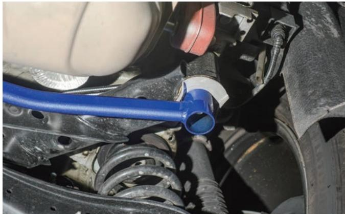
2. Install Brace to the vehicle. Then reinstall the bolts to secure the brace.
