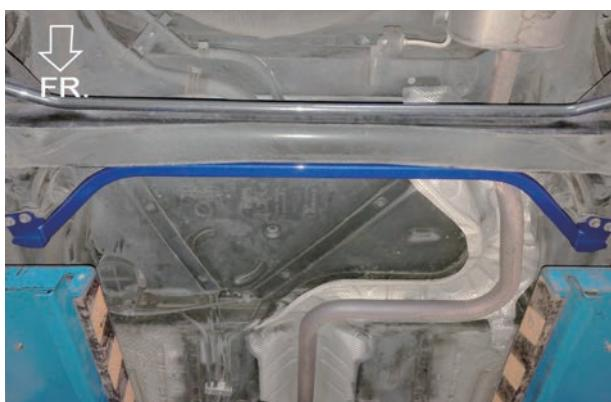
Illustration of installed state
