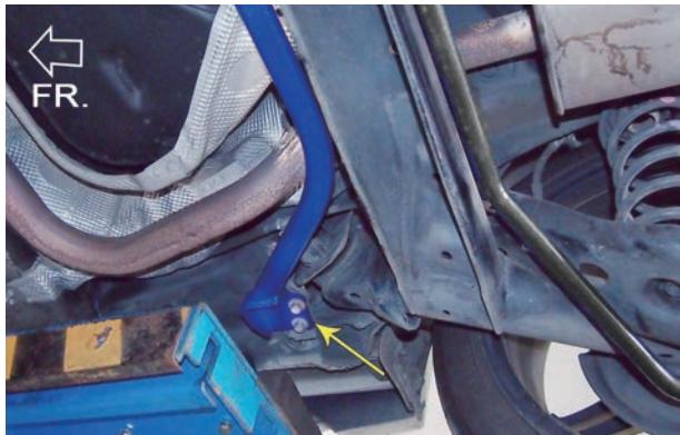
2. Place ①Brace to the vehicle and reinstall the removed bolts to secure the brace. (See figure 1&2)
