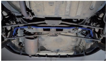
Torque for bolts 螺絲鎖緊扭力: M8-60Nm M10-80Nm M12-100Nm M14-160Nm
