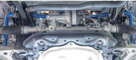
Torque for bolts 螺絲鎖緊扭力: M8-60Nm M10-80Nm M12-100Nm M14-160Nm
